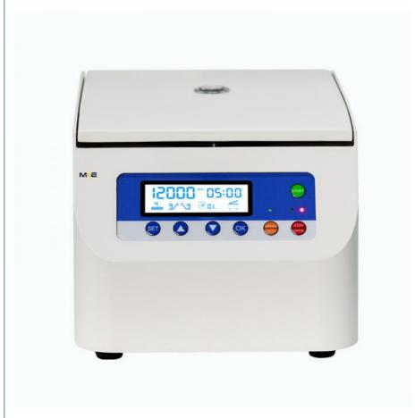
The HK-16C microcentrifuge is a versatile solution for clinical and research laboratories, offering compatibility with PCR strips, filter tubes, and 2ml–5ml microtubes. Ideal for microbiological research, protein biochemistry, and clinical chemistry, it excels in applications like sample pelleting, sedimentation, preparation, and purification.
