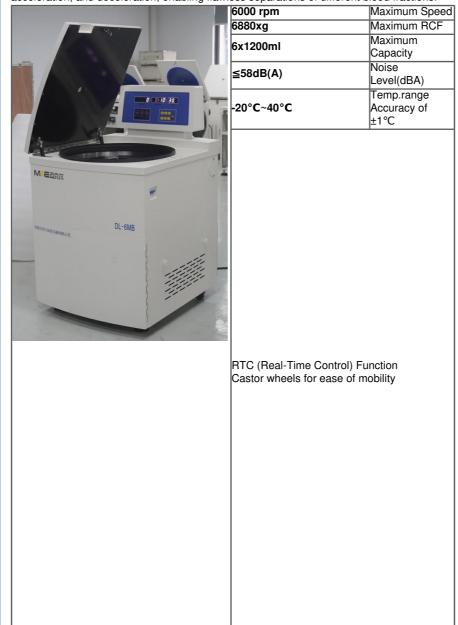
This centrifuge is highly versatile and widely utilized in blood stations, pharmaceutical facilities, biochemistry laboratories, and the production of biological products. Its applications range from essential tasks like blood separation and protein precipitation to precise cell collection, making it an indispensable asset in various scientific and medical fields.
